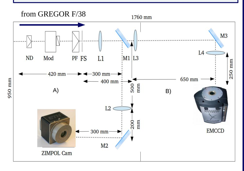
The optical setups were installed on the broad band imager table at GREGOR. The schematic layout is shown above. *FS*: science focal plane of GREGOR telescope, *Mod*: modulator based on two ferroelectric liquid crystal retarders (FLC) + a polarizing beam splitter.
