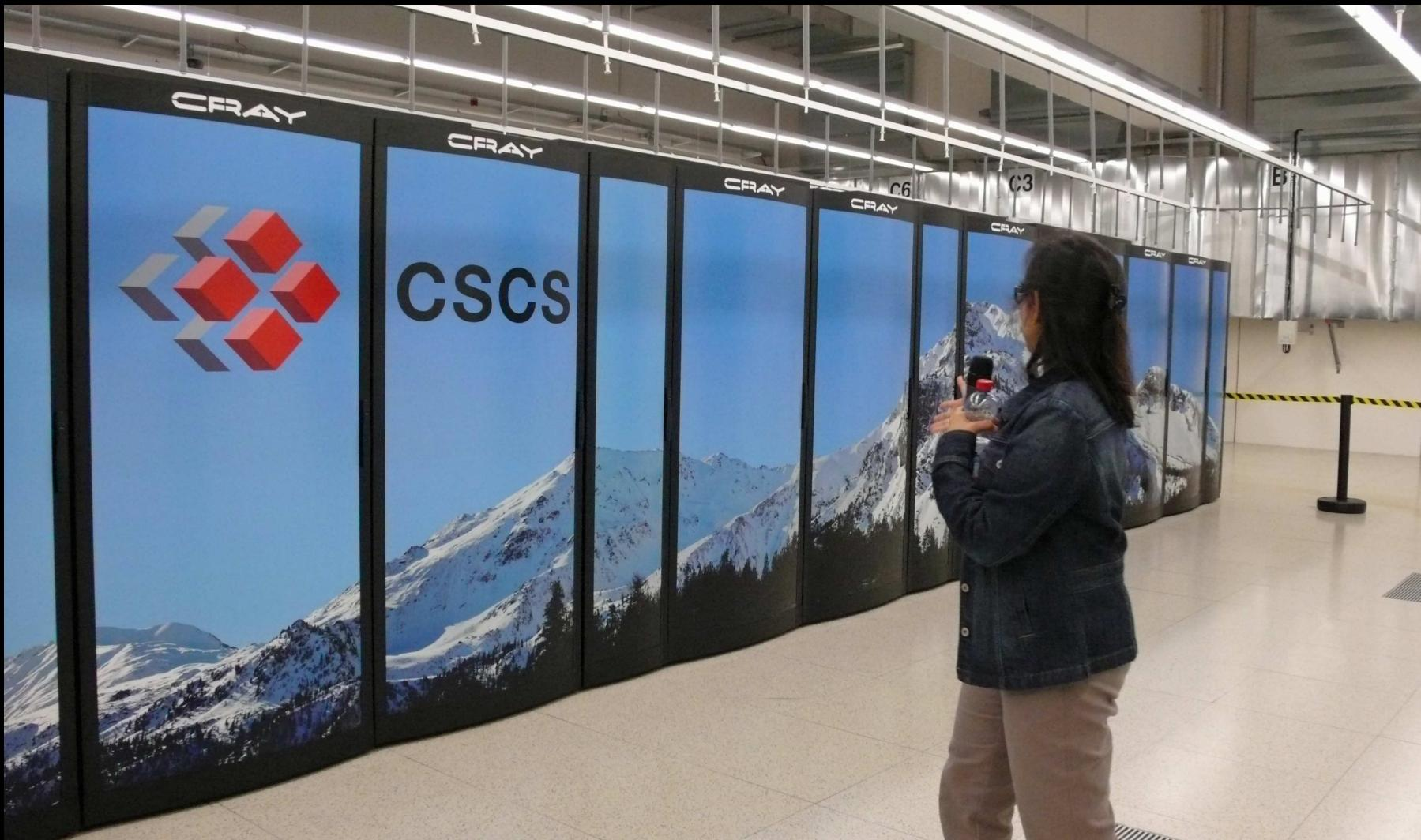
Piz Daint is a Cray XC50/XC40 with nodes of 12 cores with 64GB RAM and nodes with 18 cores and 128GB RAM, both Intel® Xeon® E5.
