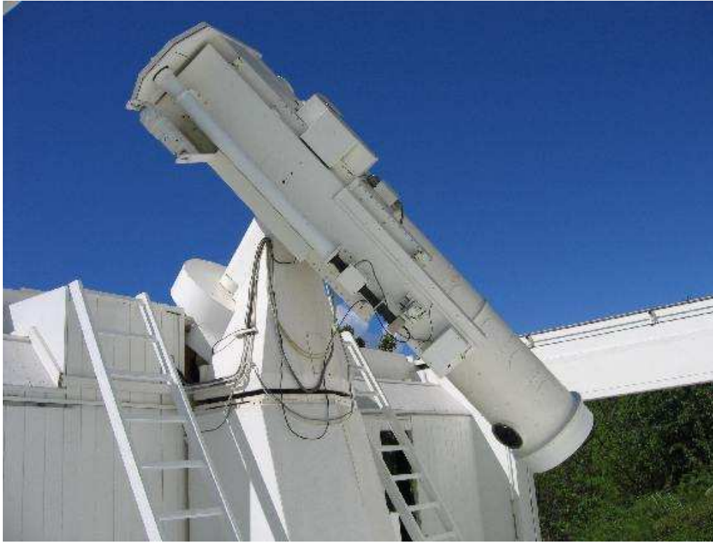
Fig. 3. The 45 cm aperture Gregory Coudé vacuum telescope.
