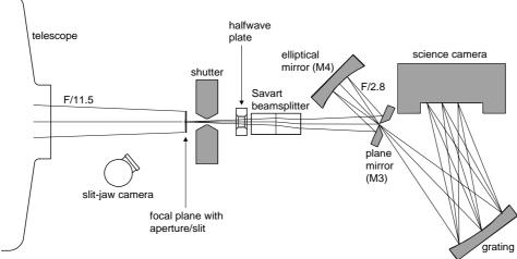
Fig. 3. Bottom: optical setup. Top left: top view of the spectropolarimeter unit. Top right: overview of the setup at the eclipse site near Waw an Namos, Libya. The spectropolarimeter unit is mounted behind the telescope. In the background one can see the tent which is used as work place and protection for the electronic equipment. The electrical power of the whole setup (150-200 W) is provided by fuel generators and secured with a UPS.
