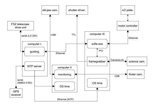
Fig. 4. Control units and programs for the eclipse instrument. The boxes with the soft edges denote computer programs, the boxes with sharp edges hardware devices. The lines of communication are annotated with the connection type and/or the protocol.
