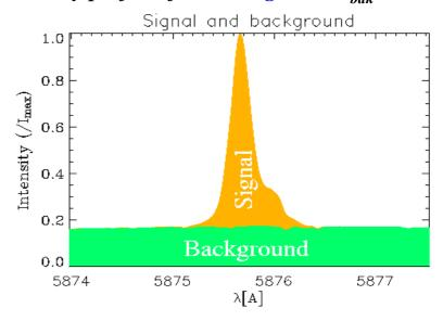
• Unfortunately we often notice a nonzero polarization outside the emission line. This has been noted to increase when the halo intensity decreases and to depend on the position on the Sun (high on NW region above solar limb). Therefore we interpret this as a spurious polarization signal from uncontrolled reflection light.
