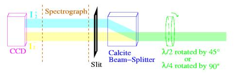
Stokes V is measured with the  $\lambda$ 4 plate.
