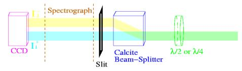
Calculation of the polarization P according to Bianda et al., 1998 A&A 331,760 allows a measurement free from effects of the detector gain table and retarder-plate transparency.
