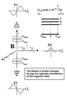
Fig. 1. The oscillator model for the Zeeman effect indicating the characteristic shapes of the circular and linear polarization profiles as generated locally via the emission process. It is important to note that the Stokes  $V(\lambda)$  profile changes its sign for opposite orientations of the magnetic field vector, while the Stokes  $Q(\lambda)$  profile reverses sign when the transverse field component is rotated by  $\pm 90^{\circ}$ .
