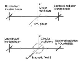
Fig. 6. The forward scattering case, in the absence (top panel) and in the presence (bottom panel) of a deterministic magnetic field.
