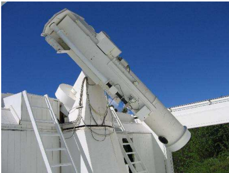
Fig. 2. The 45 cm aperture Gregory Coudé vacuum telescope.
